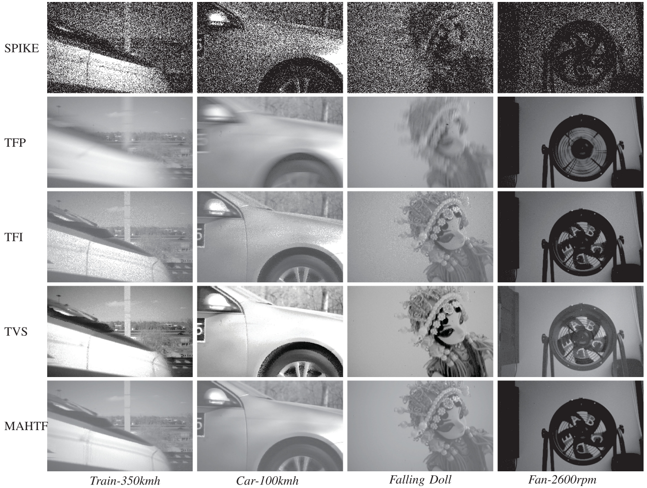
Fig. 10. Comparison of different reconstruction methods on real captured spike data. (Please enlarge the figure to observe details.) The proposed MAHTF achieves the best visual quality.
